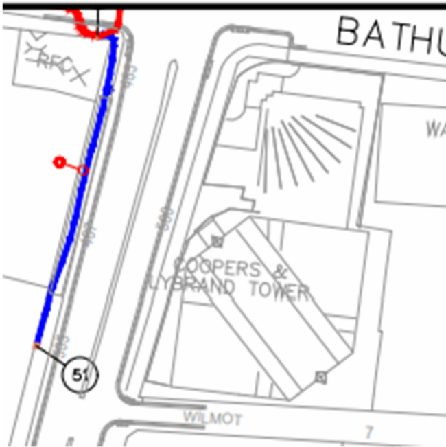
Figure 8 - Verizon Communications Services adjacent the site
